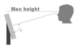
Viewing angle is an theretical value measured with standard colors and contrast. In real life the monitor should be installed with angle: 120 <  $\alpha$  < 90. This means that viewing from bottom side should be avoided. For viewing convenience install the monitor below eye-level (max height).
