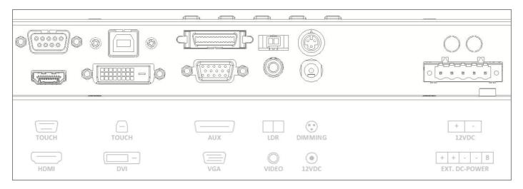
The picture above shows all connection on the I/O Bracket. For display-units with diagonal upto 12.1" the external DC-power connector counts only 2 pins, + and -:
